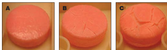
Fig. 1: Enteric coated tablets with insufficient plasticizer; (A) before dissolution test, (B) and (C) after dissolution test in the acid stage for 1 and 2 h, respectively.
