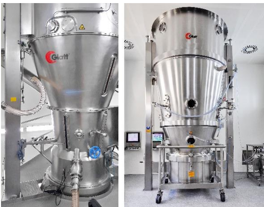
Fig. 1: Left: Fluid bed granulator with continuous product discharge; right: Batch fluid bed granulator and coater. Both systems at the Glatt Technology Center in Weimar process solvent-based products.
